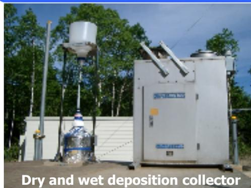
Dry and wet deposition collector
