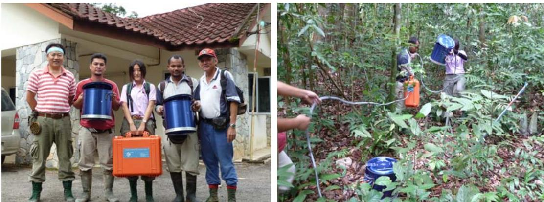
Fig. 3. A portable automated chamber system for measurement spatial variation of soil CO<sub>2</sub> efflux at different ecosystems.
